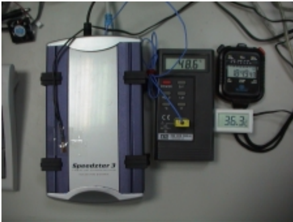
Speedster3 running 18 hour 49minute at 48.2°C
