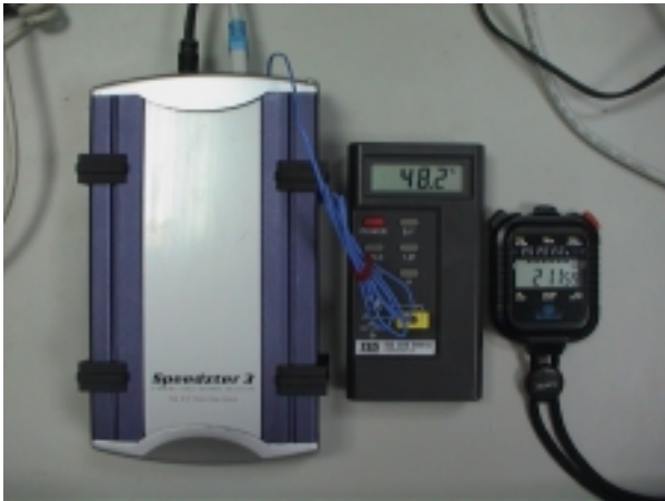
Speedster3 running 2 hour 11minute at 48.2°C
